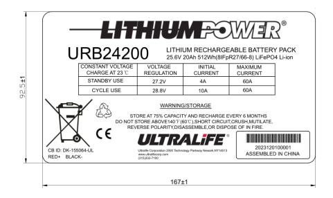
Bar Code detall: (Example:2023120100001) 20231201=YYMMDDBattery Pack Assembly Date 00001 =Battery Pack Serial Number
